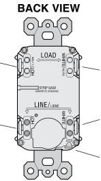
LOAD White terminal (Silver): Connection for the LOAD cable's white wire
