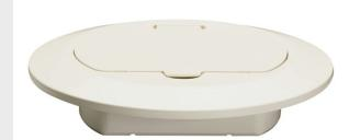
Thermoplastic Cover Includes 15 amp 125 volt Decorator receptacle, matching detachable and replacable hinged door; threaded device-mounting holes; drill guides for low-voltage poke-through holes; accepts any Decorator device; mounts on carpeting, hardwood, linoleum, tile floors; Four mounting/leveling screws. Light Almond.
