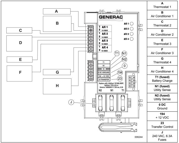
Figure 3-3. Typical SACM Connections
