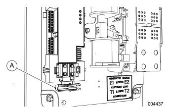
Figure 4-2. Fuse Removal and Installation Tool
