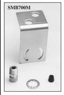
Heavy-duty 1/4-inch (6mm) zinc plated steel bracket that allows the MAXI-BEAM to retrofit to installations of MICRO-SWITCH models MLS8 or MLS9 sensors. Includes cable gland and lockwasher.
