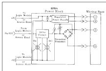
Power block models RPBA and RPBB are the most commonly used for ac MAXI-BEAM operation. As the typical hookup shows, they are intended to switch the same ac voltage as is used to power the MAXI-BEAM. However, both can switch any ac voltage that is lower than the supply voltage, as long as both ac circuits share a common neutral. Observe local codes whenever mixing ac voltages in a common wiring chamber.
