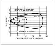
This sensor pair is designed for opposed mode operation using Banner glass fiber optics. Maximum range (HP mode) using L9 lenses is 12 feet. Maximum range using L16F lenses is 50 feet.
