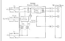
Model RPBR operates the MAXI-BEAM with either ac or dc. It offers an SPST "hard" relay contact between wiring base terminals #3 & #4, which allows the MAXI-BEAM sensor to directly interface with loads which draw high current. It also allows series connection ("AND" logic) with multiple dc sensors.
