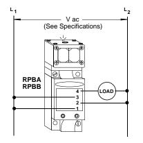
CAUTION: the output switch will be destroyed if the load is shorted.
