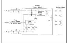
RPBR2 is an SPDT output version of model RPBR, with both contacts common to terminal #1. Terminal #3 is normally open; terminal #4 is normally closed. See application caution, page 9.
