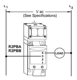
MAXI-BEAM sensors using power block R2PBA or R2PBB wire in series with an appropriate load. This combination, in turn, wires directly across the ac line. A 2-wire sensor may be connected exactly like a mechanical limit switch.
