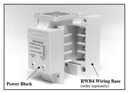
MAXI-BEAM power blocks provide regulated low voltage dc power to the sensor head and logic module (if one is used), and all power blocks (except emitter-only types) contain an output switch for interfacing to loads or to control circuitry.
