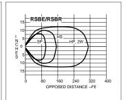
MAXI-BEAM emitters have a visible red "tracer beam". This beam is non-active, and is used as a means of visual alignment during installation. A retroreflector temporarily attached to the receiver lens provides an effective target for the tracer beam during alignment. The narrow beam of the RSBESR/RSBRSR pair is ideal for sensing small parts (effective beam diameter is 0.14 inch).
