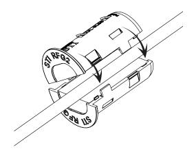
Install grommet halves around cable(s), teeth of grommets interlock securing grommet halves together.
