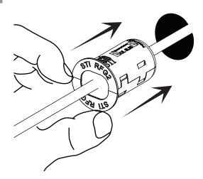
Slide grommet down cable(s) into opening until faceplate abuts wall surface.
