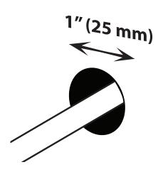
Cut nom. 1" (25 mm) diameter opening into gypsum board wall and run cable(s) through opening.
