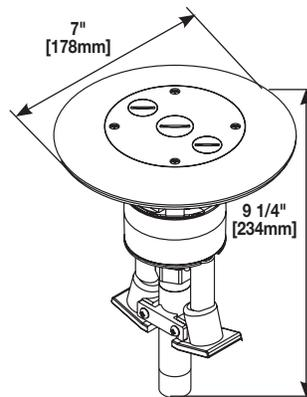
**NOTE:** For installations in the City of Chicago, install an EMT compression fitting (not supplied) to the conduit system and a junction box suitable for use in environmental air spaces, if required, (not supplied). Complete installation per NEC and local codes.
