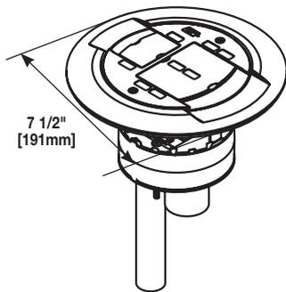
**NOTE:** For installations in the City of Chicago, install an EMT compression fitting (not supplied) to the conduit system and a junction box suitable for use in environmental air spaces, if required, (not supplied). Complete installation per NEC and local codes.
