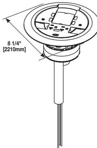
**NOTE:** For installations in the City of Chicago, install an EMT compression fitting (not supplied) to the conduit system and a junction box suitable for use in environmental air spaces, if required, (not supplied). Complete installation per NEC and local codes.
