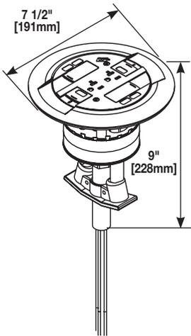
**Assembled Unit** – Prewired 20A duplex receptacle can be wired as standard duplex or isolated ground. Wiremold Open System unloaded inserts to accept four discrete keystone connectors from most manufacturers are provided.
