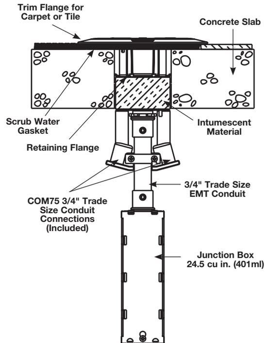
**CAUTION:** These devices are suitable for 1, 1 1/2, and 2 hour rated floor assemblies as described in the UL Fire Resistance directory for each service. These devices meet all UL scrub water requirements, but are not suitable for wet or damp locations, or other areas subject to saturation with water or other liquids such as commercial kitchens.
