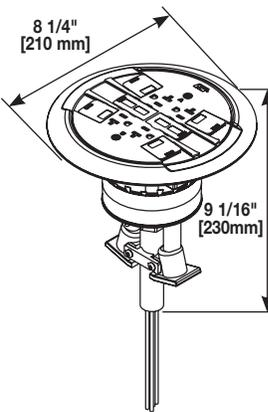
**Assembled Unit** – Unit includes four prewired 20A receptacles. Each duplex can be wired as a separate circuit. The duplex can be wired as a standard receptacle or isolated ground. Wiremold Open System unloaded inserts to accept four discrete keystone \* connectors from most manufacturers are provided.
