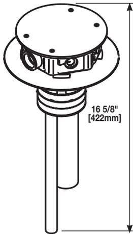
**Assembled Furniture Feed Unit –** Complete with hexagonal service head. Service head has one 3/4" threaded conduit hub and five rubber grommets. The service head includes scrub water gasket. Unit is supplied with one 1 1/4" trade size conduit stem and one 1/2" trade size conduit stem to feed power and communication services.
