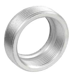
1" to 3/4" reducing bushings are used with threaded rigid or IMC conduits to reduce the size of female hubs in order to accommodate smaller sized conduits or male threaded hubs. Garvin Industries' stainlesssteel construction maintains mechanical protection and solid grounding of the conduit to the designated electrical junction box or enclosure. These reducing bushings are stainless steel for excellent corrosion protection in wet or damp locations.
