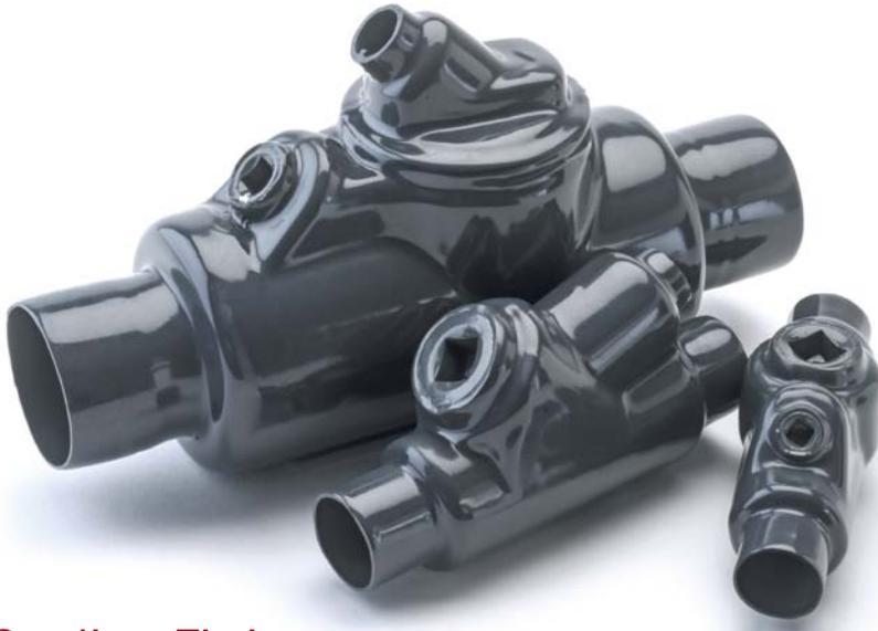
*These Plasti-Bond REDH<sub>2</sub>OT sealing fittings should be used with a suitable system of sealing compound, such as Chico A, Chico X or Chico A-P from Crouse-Hinds. Follow the installation instructions included with the sealing compound.*
