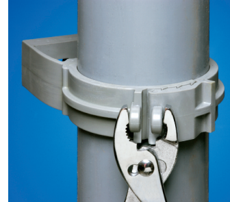
2-1/2" - 4" Press pipe into QuickLATCH, up to the first notch to lock it in place. Finish by squeezing tabs together for a super-secure hold.
