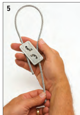
5 To adjust, remove tension and pull wire rope slightly to disengage teeth, slide adjustment pin in direction shown by arrow to release wire rope.
