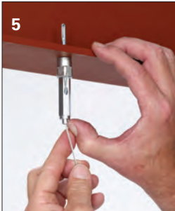
5 To adjust down - push up on bottom of KwikWire Hanger and allow cable wire to feed down
