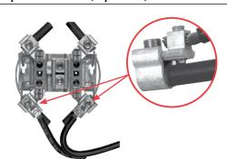
Replaces the load or line side slide-in nut assembly on Milbank 200 amp sockets. Allows for a 100 amp tap location in addition to the #6-350 kcmil load-side connector. **K5022** includes safety barrier extensions for applications over 300 VAC. Three lugs per kit.
