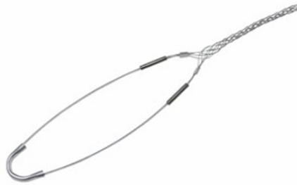
Bus drop, Closed mesh, Single eye. Cable diameter - 9", Mesh length - 3.5", Break strength - 1,100 lbs.
