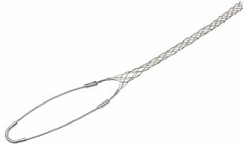
Standard-duty, Closed Mesh, Single eye grip. Cable Diameter - .0500-.0610", Bale length, 7", Mesh length, 11", Break strength, 770 lbs.
