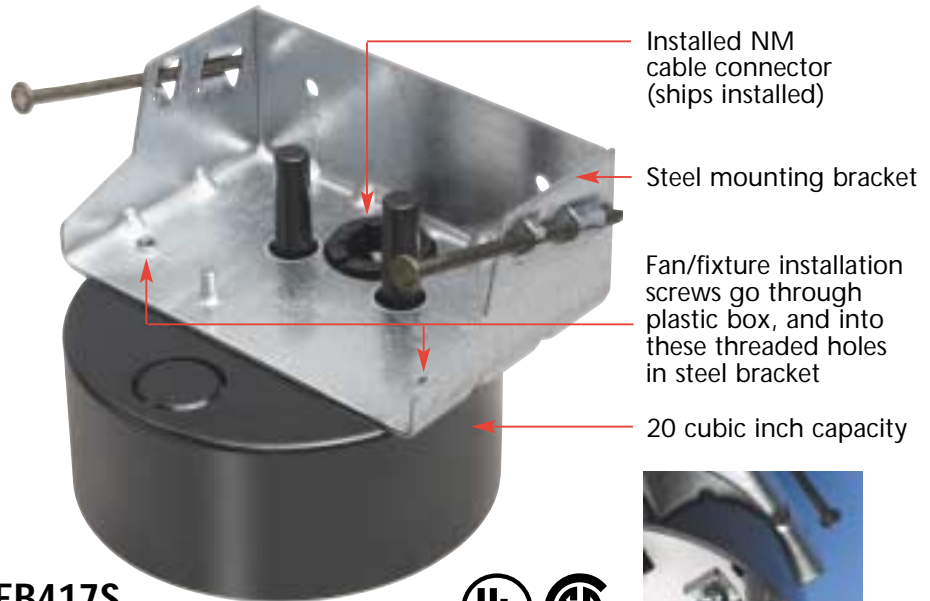
FB417S Plastic Box with Steel Bracket
