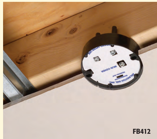
1 The FB412 fan/fixture box is perfect for 1/2" or 5/8" drywall with 3/4" furring strips or hat channel with a single layer of drywall...
