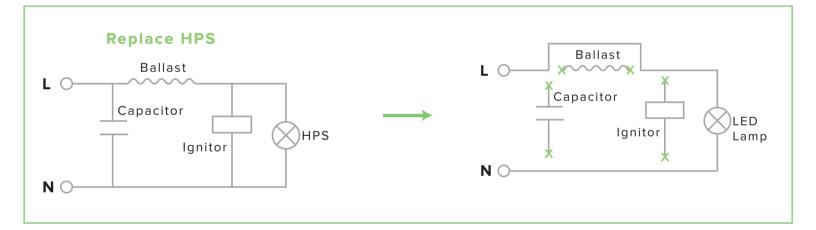
**STEP 3:** Be sure to remove the existing ballast if there is one and discard according to local laws and regulations. Please see proper wiring diagram above.
