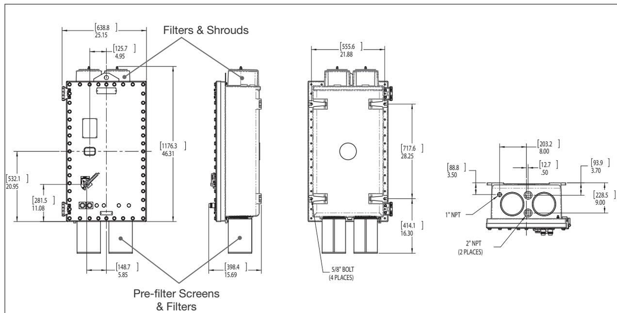
Enclosure Size 2 (7.5 to 50.0 Horsepower VFDs)
