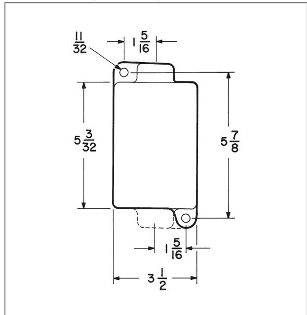
**Note:** Depth is 5.5" from front of switch to back of box.
