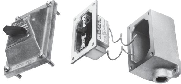
EDS factory sealed snap switches or manual motor starting switches do not need external sealing. The switches are enclosed in a unique sealing well with double flanges which mate with the cover and the body. Small, compact enclosures have accurately ground wide flanges on body, cover and sealing well for flame-tight joints. Wiring pigtails are factory sealed from under the sealing well. Reliable pouring of seals at the factory ensures safe sealing.
