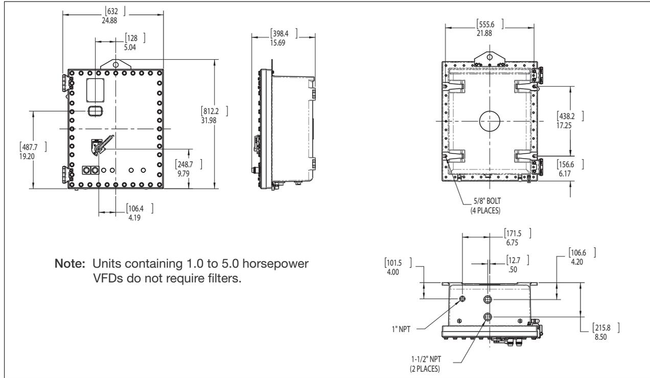
Enclosure Size 1 (1.0 to 5.0 Horsepower VFDs)
