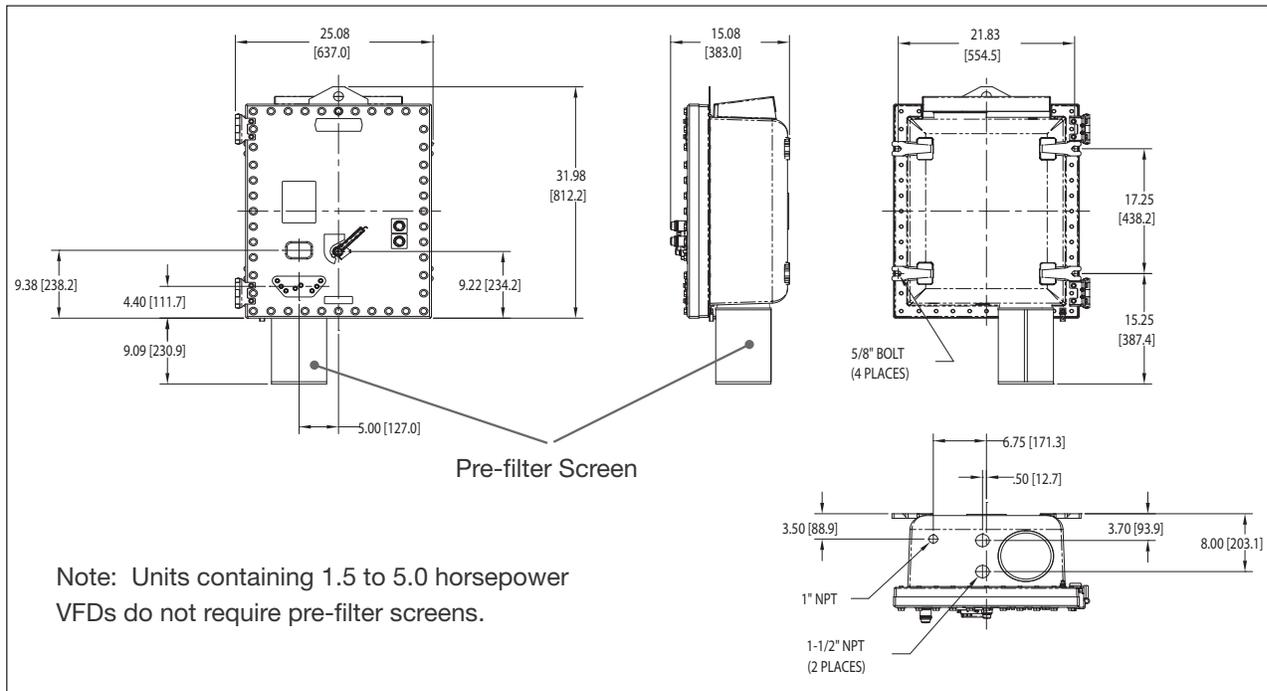
Enclosure Size 1 (1.5 to 10.0 Horsepower VFDs)
