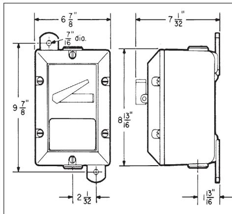
†Enclosures are furnished with two 1/4" drilled and tapped openings with 1/4" to 1" reducers.
