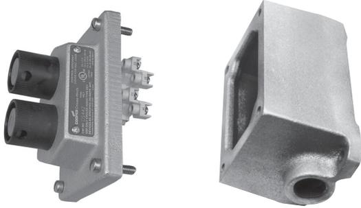
Factory sealed EDS and EFS pilot light, pushbutton and selector switch control stations do not need external sealing. Device contacts are factory sealed in explosionproof ESWP contact blocks. Small, compact enclosures have accurately ground wide flanges on both the body and cover for a flame-tight joint.
