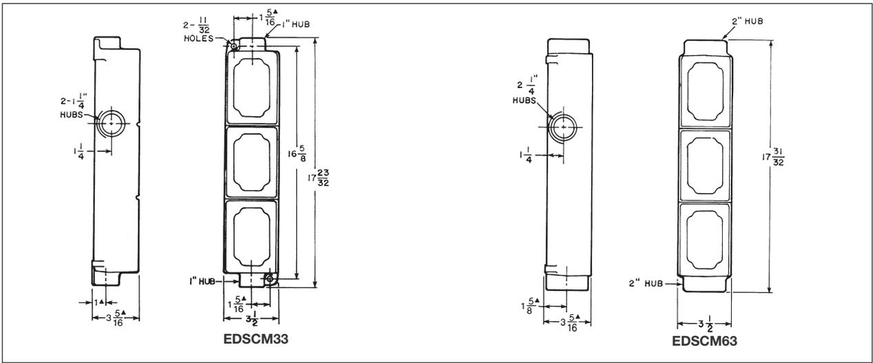
\* When a CPS receptacle cover device is used, the assembly meets requirements for Class I, Groups C and D areas only. Dimensions are approximate. Not for construction purposes.
