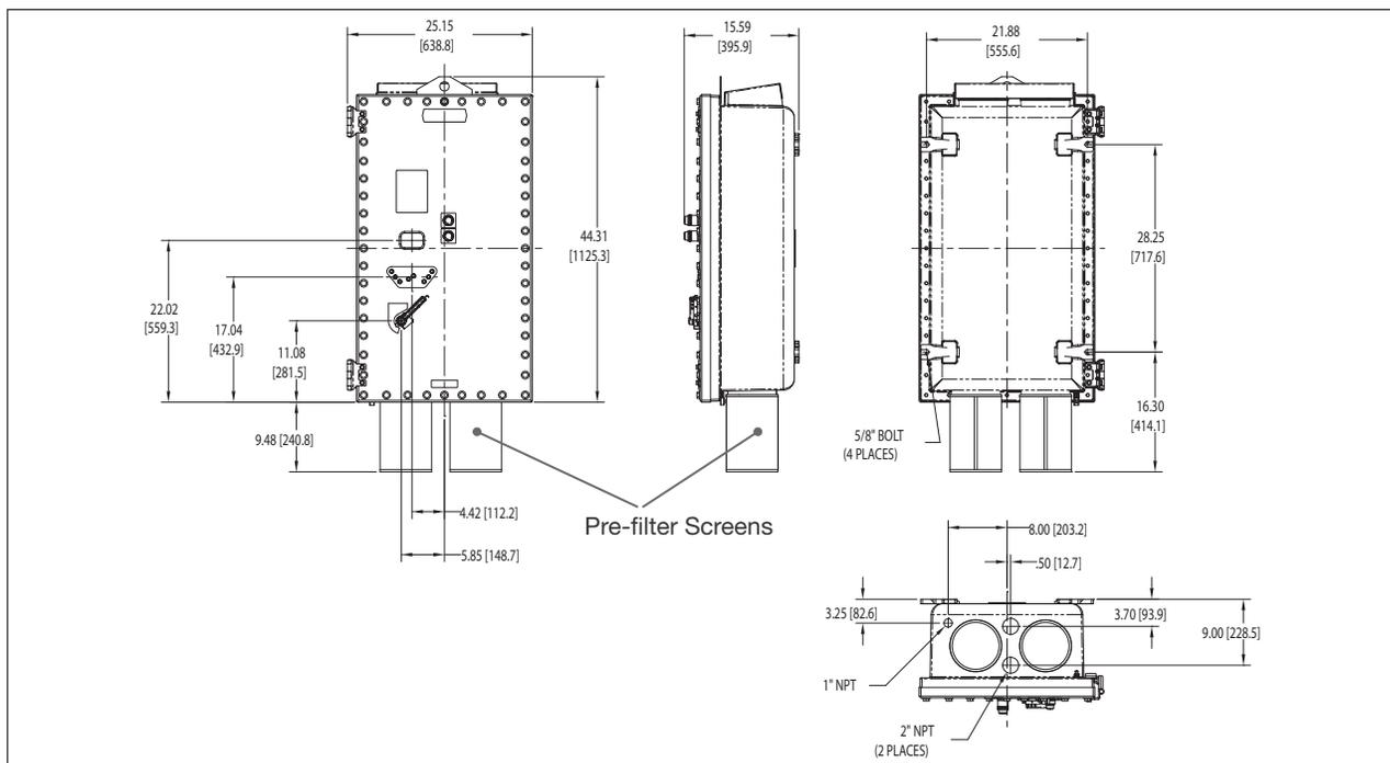
Enclosure Size 2 (15.0 to 60.0 Horsepower VFDs)
