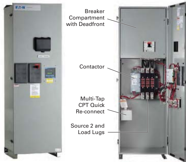
225-400 A Service Entrance Contactor NEMA 1
