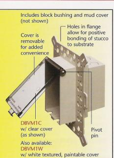
Meets 2005 NEC, Section 406-8 For the protection of exterior outlets which require the use of a weatherproof-in-use cover for all outdoor 15 or 20 amp receptacles.
