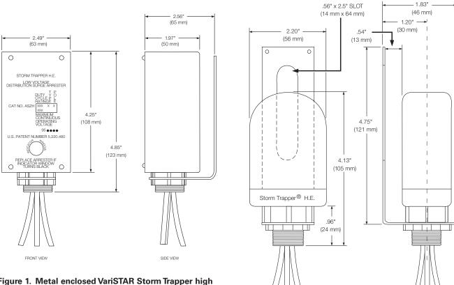
Figure 1. Metal enclosed VariSTAR Storm Trapper high energy MOV arrester with optional mounting bracket.
