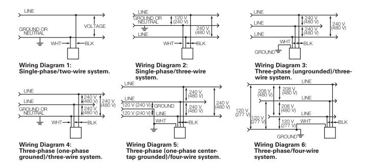
Figure 3. Wiring diagrams.
