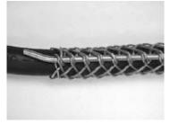
3. To remove the grip, pull the rod out
