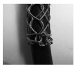
4. Wrap the laces tightly around the tail of the grip once or twice. Twist the ends tightly to secure. Extra lace may be cut off
