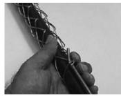
Place the grip around the cable. Starting at the eye end, thread the rod through the formed loops with a corkscrew motion. Use the curved leading end of the rod to pull the loops together
