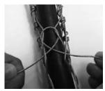
Place the grip around the cable. Starting at the eye end, thread the lace through the first two loops on either side of the mesh split. Pull the lace through the loops until the lace strands and thread them through the next two loops. Continue lacing the grip with this method
