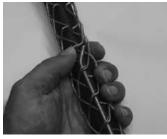
2. Use a steady push and twist motion with the hand on the rod. The fingers of the other hand pull the mesh loops together in front of the leading end of the rod
