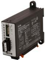
Modbus with I/O Module
