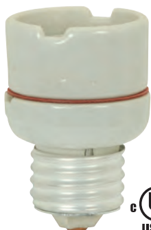
90-2589 Medium to Medium E26 - E26 2 Piece Glazed Porcelain Extender Overall Ext. 1 1/4" 660W-250V
