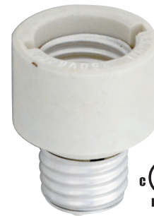
92-324 Medium to Medium E26 - E26 Extender Porcelain Overall Ext. 1" 660W-250V
