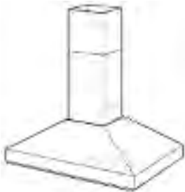
8" Round Duct — Internal Blower 900 CFM, 9.5 Sones 8" Round Duct — External Blower 280 – 1500 CFM
