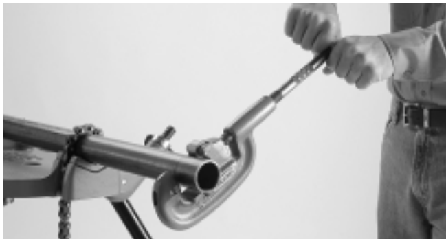
Figure 1 – Cutting End of Pipe
