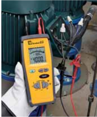
Tests insulation on motor windings
