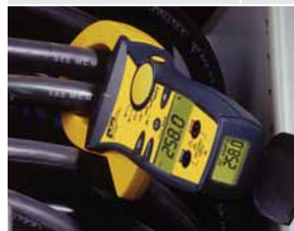
Large jaws for clamping around multiple conductors
