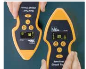
Display rotates in 90° increments so that you always receive an upright reading.
