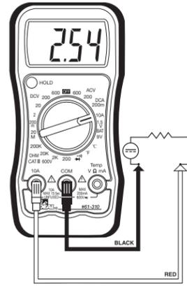
Turn power off, break circuit, insert meter in series, then turn power back on.
