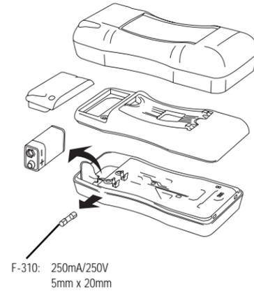
**WARNING:** To avoid electric shock, disconnect test leads before removing battery cover.
