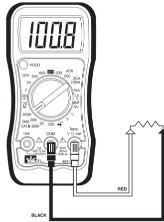
**WARNING:** De-energize circuit before taking resistance measurement.
