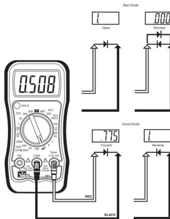
**WARNING:** De-energize circuit before checking diode.
