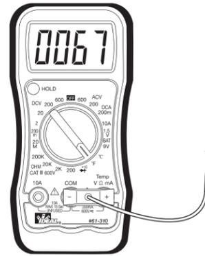
**WARNING:** To avoid electric shock, do not place test leads or thermocouple on a voltage source.
