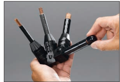
6. Reapply end nut and tighten.
