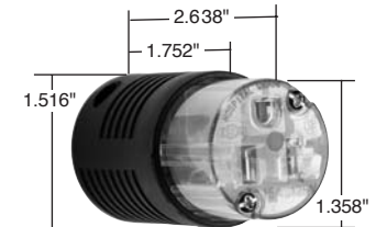
Dimensions for 15 & 20 Amp Connector
