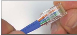
Insert wire pairs into plug
