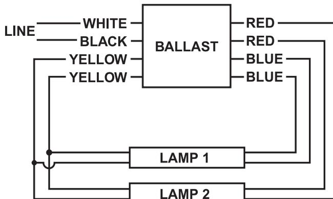
**MOUNT LAMPS WITHIN 1 OF GROUNDED METAL REFLECTOR**
