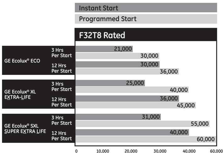
Life ratings are based on engineering data on programmed start ballasts with lamps cycled every 3 operating hours.
