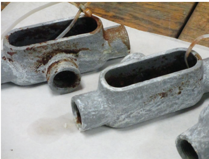
Representative samples of old Duraloy ® paint after 1,000 hours of exposure
