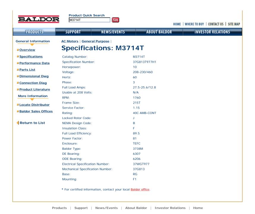
Products: AC Motors: M3714T: Baldor Electric Company, a leader in energy efficient electric motors, linear motors and adjust... Page 2 of 2
